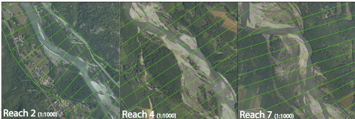
Figure 2.11 Orthophotos of reach 2, sinuous single thread, and reaches 4 and 7, wandering type (scale 1:1000). Green lines plot the DGO sequences.
